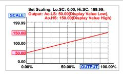
The range between Ao.HS and Ao.LS should be over 20% of span at least; otherwise, it will be got less resolution of analogue output.
