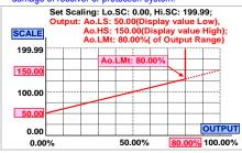
Fine zero & span adjustment:
