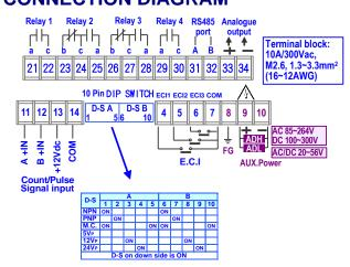
Please check the voltage of power supplied first, and then connect to the specified terminals. It is recommended that power supplied to the meter be protected by a fuse or circuit breaker
