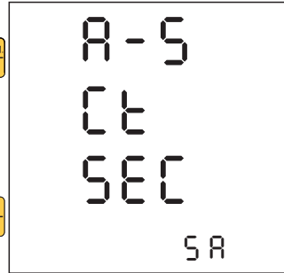
Current setting of CT secondary side 1A/5A
